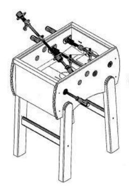
Place the rods into the holes from the handles side.
