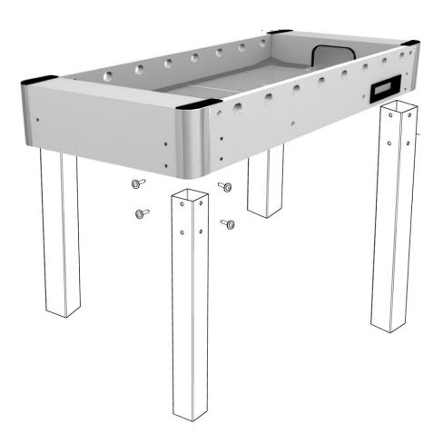
Assemble and fix all 4 legs with their metal flat and screw (8x45 ) by using the Allen spanner key (5)
