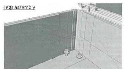
Insert the pin of the leg inside the holes
