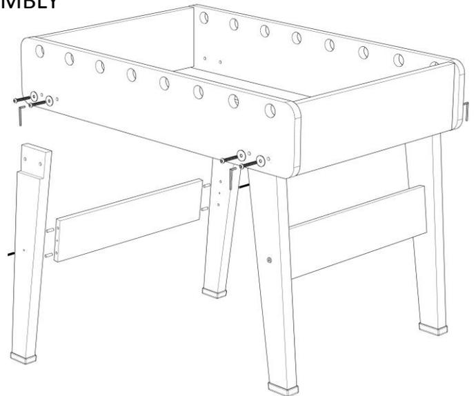
Place the Pin diam.10 in the crossbar and fix the legs using the allen sparn 4mm with the screw 8x55
